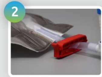
Clamp the bag tubing below the sample port with the red clamp
